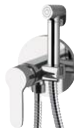
W 65 W Built-in shower mixer set including shut-off art. 332OW, shower holder water punch on flange, all in c.p. brass, with 1/2 connection, hand shower support and shower flexible cm 120.
