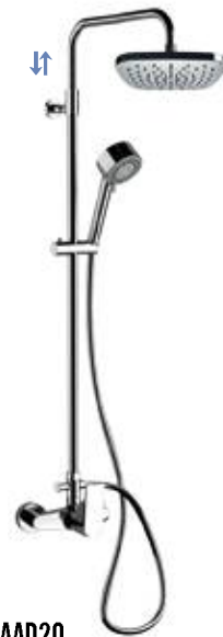
D 37 AAD20 CR € 411,80 Shower mixer with upper 3/4" connection, with telescopic shower column, c.p. hand shower 4 functions antilimestone, with 333 CNX 150 cm flexible hose and c.p. ABS squared with rounded corners shower head, rain jet Art. 356 AD 20, 20x20 cm, with anti-limestone silicon jets.
