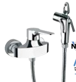
WC 31 DP Wall mounted single-lever shower mixer, interaxis 100 mm, with kit composed by shut-off hand shower in c.p. abs art. 332DPCR, conical flexible in c.p. brass cm 120 and c.p. hook art. 332GA.
